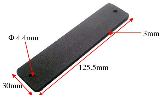
Note: Tolerance applicable are **Length:**  $\pm 1\text{mm}$ , **Width:**  $\pm 0.5\text{mm}$  and **Thickness:**  $\pm 0.3\text{mm}$ .
