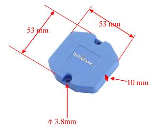
Note: Tolerance applicable are Length: ±1mm, Width: ±0.5mm and Thickness: ±0.3mm
